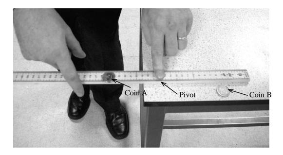
A coin, A, is placed on top of the smooth ruler and another coin, B, is placed on the table.
