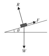
(i) State expressions for the components of the weight of the box parallel to the back of the lorry and perpendicular to the back of the lorry.
